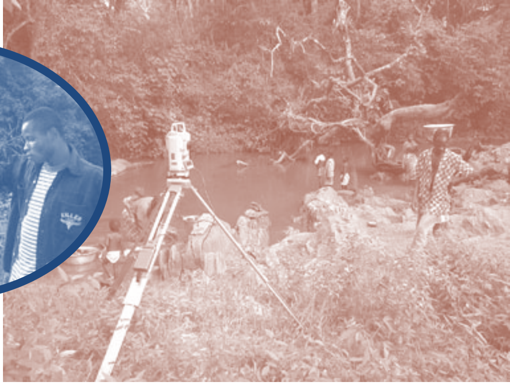
Preliminary survey to evaluate suitable sites for SHP in remote areas without electricity generation, Togo. (© Studio Frosio)
