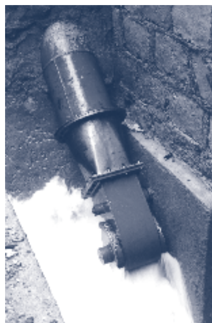
5kW crossflow turbine, India. (© IT Power)
