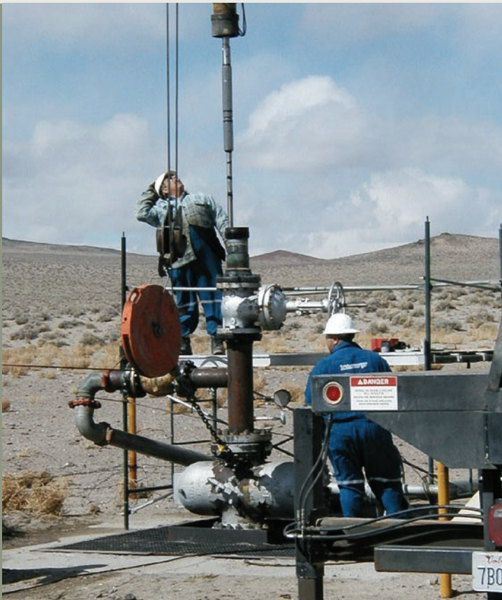
Drilling exploration crew performing initial well logging tests at the Desert Peak site in Nevada.
